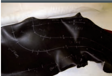
5 Make sure that you mark your pattern with enough information. Color, seam allowances, sew foam, and in some cases the direction the patterns have to be placed on the material.
