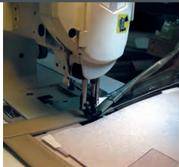
9 Two views of the large binder at work. Note the white 3/4-inch line and the binder finishing to the edge of the line. The finished binder width is 1 1/2 inches, so 3/4 inch of this width is off the edge of the glass on the top and sides of the panel being worked on in these two pictures.
