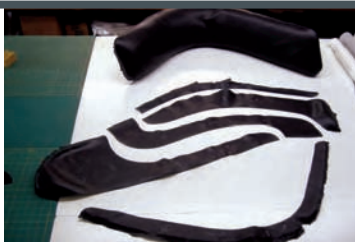
6 The old vinyl has been cut apart and is ready to use as the patterns.
