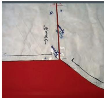
1 One of our Tyvek patterns off the boat and developed to the point that we can start cutting the Strataglass and Sunbrella we use in 90 percent of our fabrications. Notice that the bottom edge and start and stop points of the top zippers are marked on the pattern, as well as one corner division between two adjacent panels. (I'll explain these down-turned corners in a future article on natural intersections and patterning.) We cut the pattern up 3/4 inch from the bottom edge of each top zipper.
