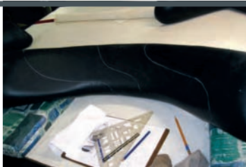
4 Once a design has been selected, if the vinyl is still intact, draw it out before you remove the vinyl from the cushion.
