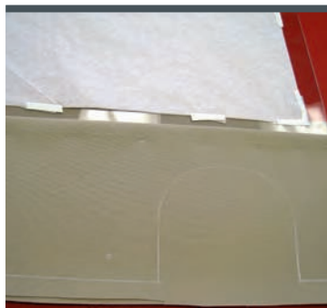
4 Add 3/4-inch double-sided seam tape to the bottom edge of each side of the vinyl glass. Fold the bottom fabric on the 3/4-inch line, remove the backing of the seam tape and slide up onto the glass and stick. The bottom of the vinyl glass panel should line up with the punched hole line on the fabric.
