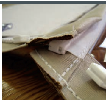
14 A close-up view of the vertical zipper overlap. If you removed the vertical binding, the two edges of the raw glass would butt each other. mf
