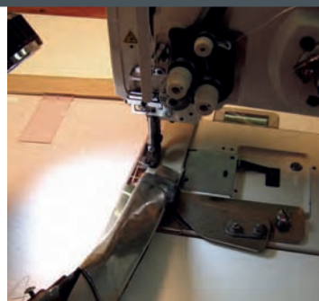
9 Two views of the large binder at work. Note the white 3/4-inch line and the binder finishing to the edge of the line. The finished binder width is 1 1/2 inches, so 3/4 inch of this width is off the edge of the glass on the top and sides of the panel being worked on in these two pictures.
