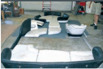
1 The old upholstery removed from the boat and laid out on the shop floor.
