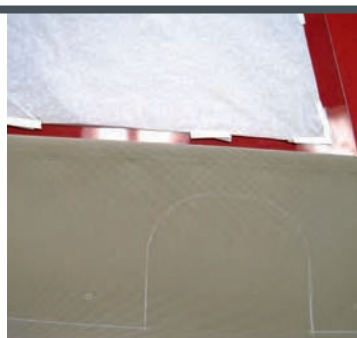
5 Flip the panel over, remove the backing of the double-sided tape, fold and stick the top of the bottom fabric to match the folded edge on the front side.
