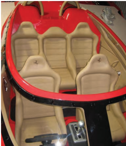
A high-performance boat was presented to this fabricator as a fiberglass shell with the request to fabricate an interior mimicking a F-440 Ferrari car. When the potential job you're creating an estimate for includes custom elements, remember to factor in design time. Photo: VIP Upholstery & Interior Design LLC, St. Peters, Mo.
